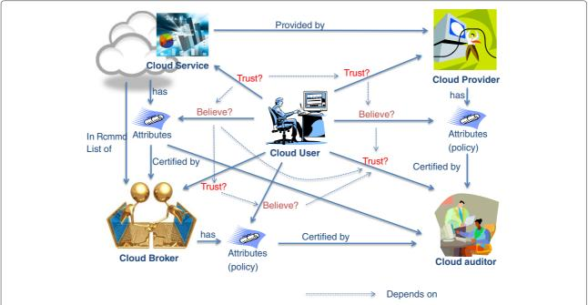
**Figure 7 Chains of trust relations in clouds.** This figure provides an integrated picture to illustrate the chains of trust relations from a cloud user to a cloud service and related cloud entities, where accreditation is omitted for simplicity.
