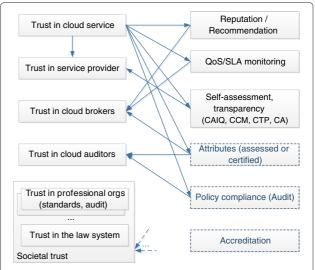
**Figure 6 Evidence and chains for trust judgment on a cloud service.** Trust placed in a cloud service is based on one or more of: (1) cloud service provider, whom is trusted; (2) policy compliance; (3) certified attributes; (4) QoS monitoring and SLA verification, which are conducted by a trusted party such as a trusted broker; (5) reputation calculated or recommendation made by a trusted broker.
