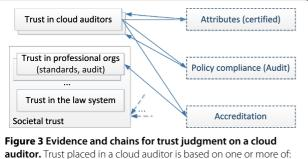
**Figure 3 Evidence and chains for trust judgment on a cloud auditor.** Trust placed in a cloud auditor is based on one or more of: (1) accreditation, which is further based on the trust placed on professional organizations making standards and audit/accreditation, – a part of societal trust; (2) policy compliance, which is audited by another trusted auditor; (3) attributes, certified by another trusted auditor.
