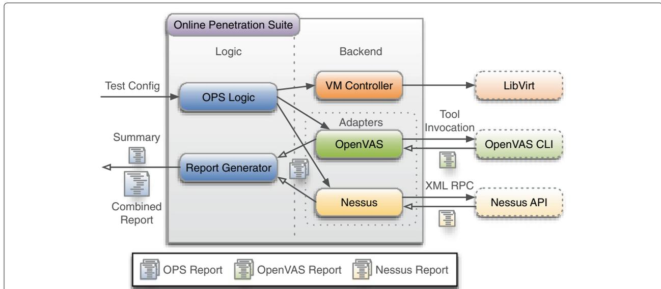
**Figure 3 Online Penetration Suite architecture.** The architecture of the Online Penetration Suite.
