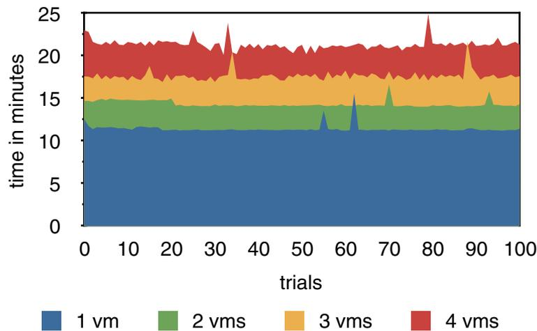
**Figure 7 Results of the OPS evaluation.** Benchmark of the runtime of the OPS depending on the number of tested systems.
