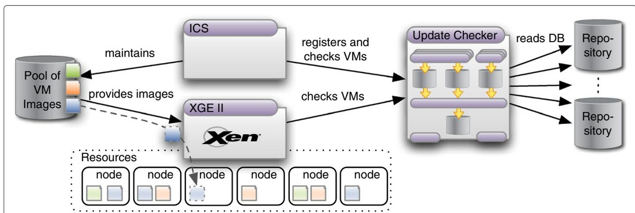
**Figure 2 Usage scenario.** The architecture of a complete system for virtualized Grid computing, consisting of the ICS, the XGE and the Update Checker. The figure shows the XGE deploying and starting a virtual machine, after the Update Checker has attested the virtual machine as being up-to-date.
