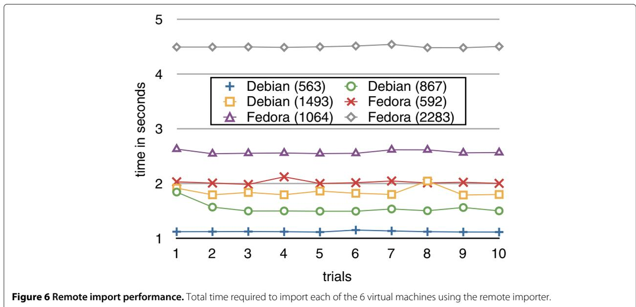
**Figure 6 Remote import performance.** Total time required to import each of the 6 virtual machines using the remote importer.
