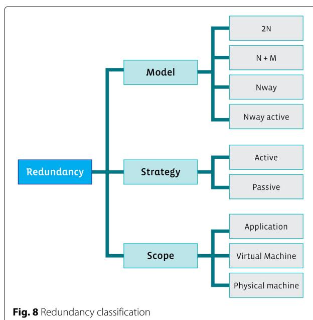
**Fig. 8** Redundancy classification
