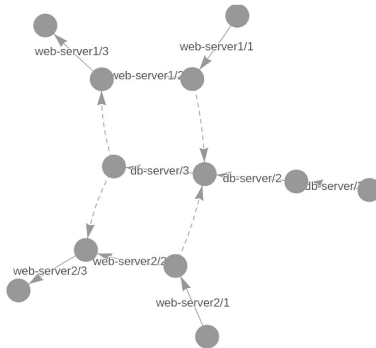
**Fig. 3** Wordpress deployment graph with 2 Web Servers and 1 Database Server
