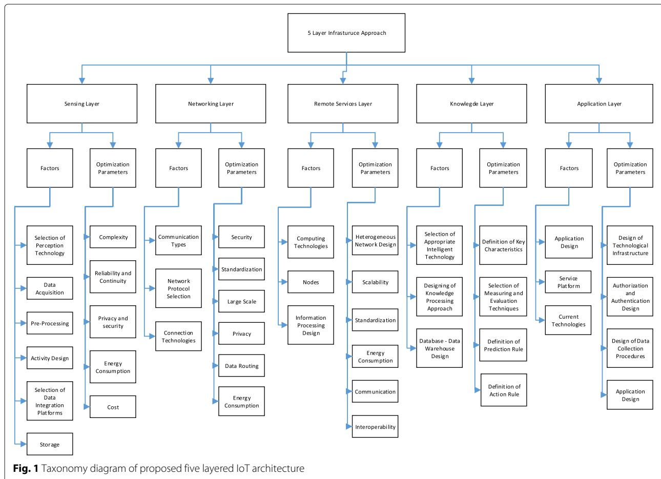
**Fig. 1** Taxonomy diagram of proposed five layered IoT architecture
