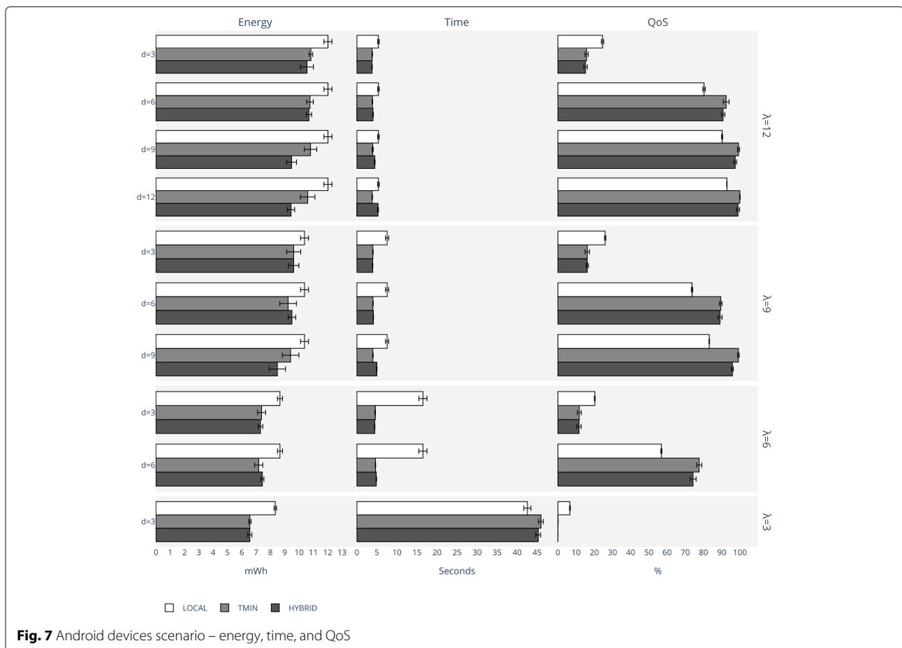
Fig. 7 Android devices scenario – energy, time, and QoS
