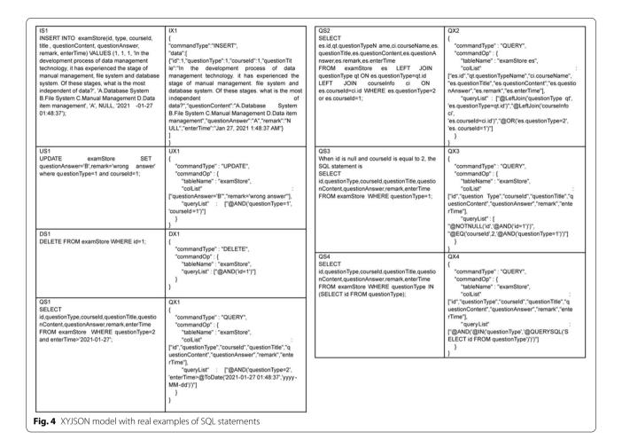
@EQ implies that when the course Id is equal to 2, the query condition with question Type = 1 will be used. @ AND indicates that multiple query criteria are connected by "AND."
