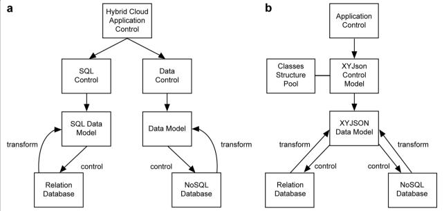
Fig. 1 Comparison of XYJSON and traditional hybrid database control structures (a) Traditional hybrid database control structure (b) XYJSON hybrid database control structure
