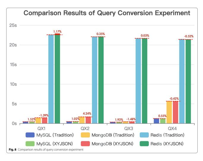
realized the modification and deletion of different types of databases using one command mode, and in the relational data and MongoDB database, the modification performance was slightly better than that of the traditional model, and the gap between other operation performances was small.
