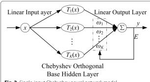
Fig. 2 Single-input Chebyshev neural network model
