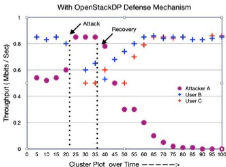
Fig. 35 Throughput Performance during Insider Attacks
