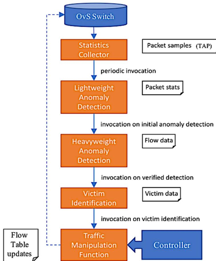
**Fig. 13** High-level workflow of network anomaly detection
