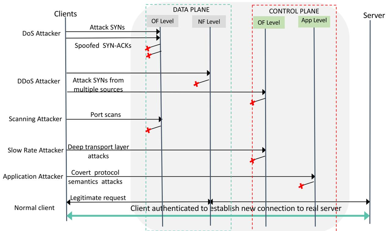
**Fig. 33** Depth traveled by attack traffic in the pipeline
