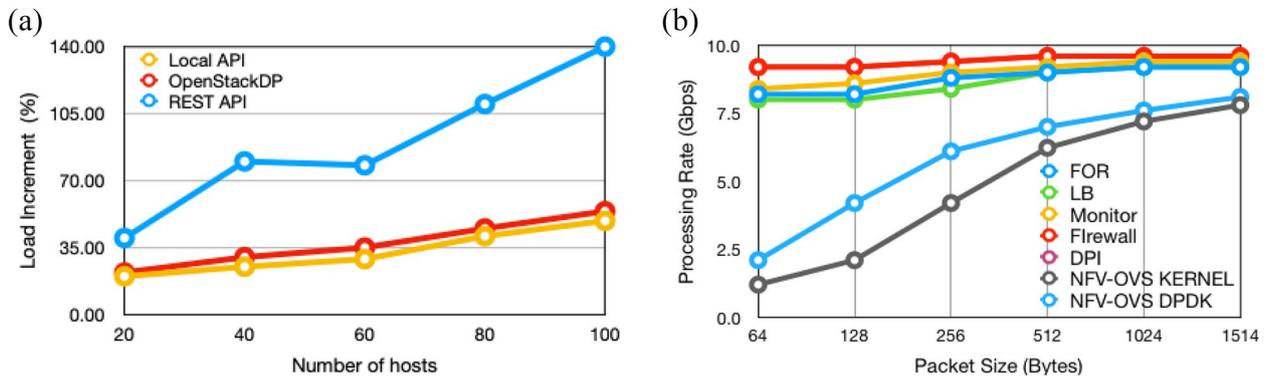
Fig. 26 a OpenStackDP API Scaling b NFV Throughput
