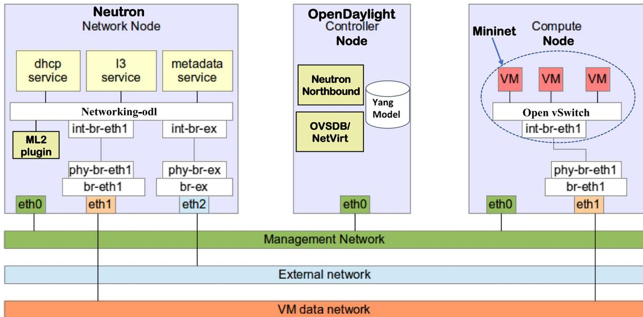
Fig. 19 OpenStackDP Testbed Environment
