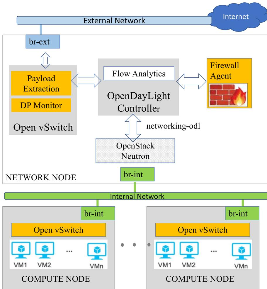
**Fig. 7** Intelligent SDN-based Firewall in Network Node
