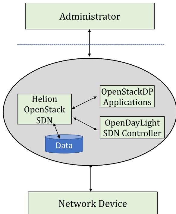
Fig. 36 DFD for OpenStackDP Framework
