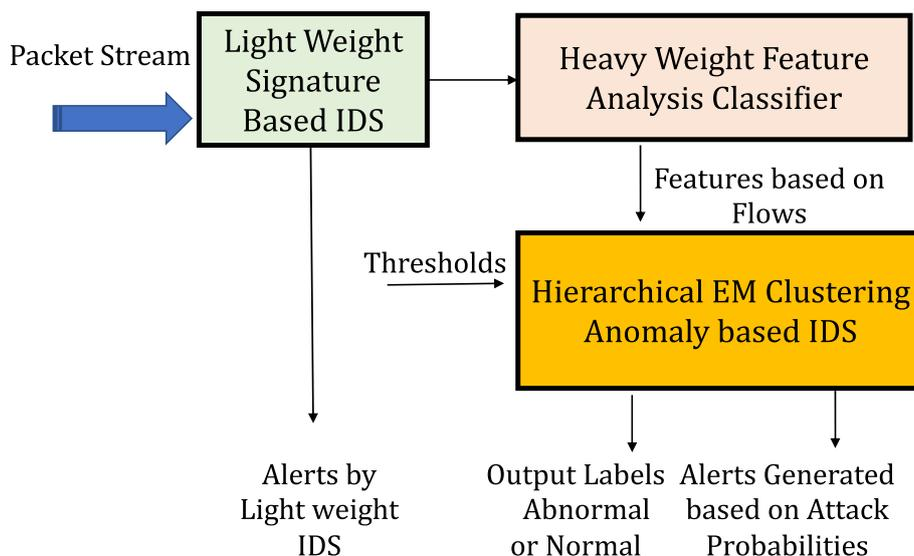
Fig. 11 General Architecture of Anomaly IDS
