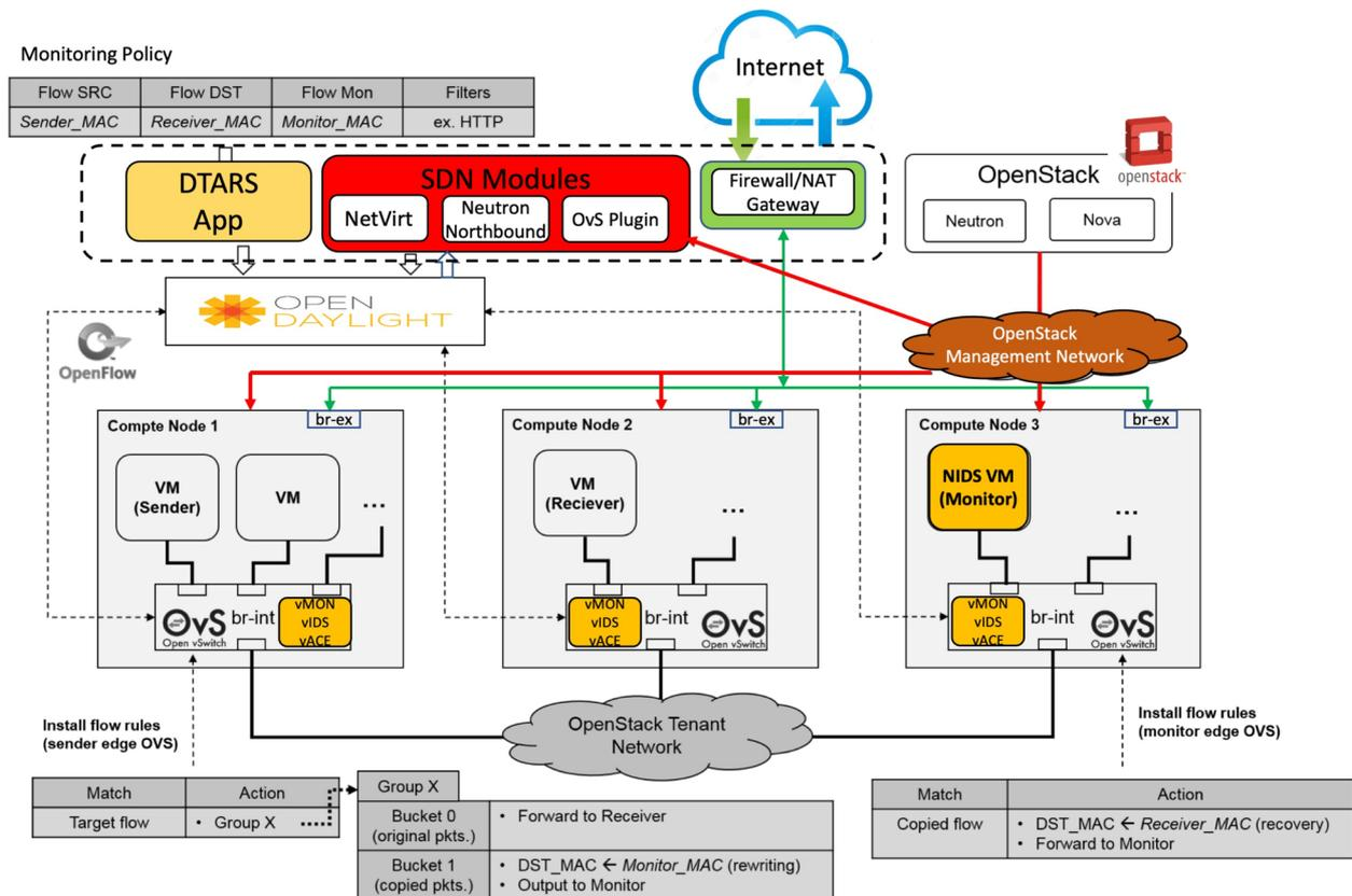
Fig. 6 SDN-enabled OpenStack Architecture (OpenStackDP)
