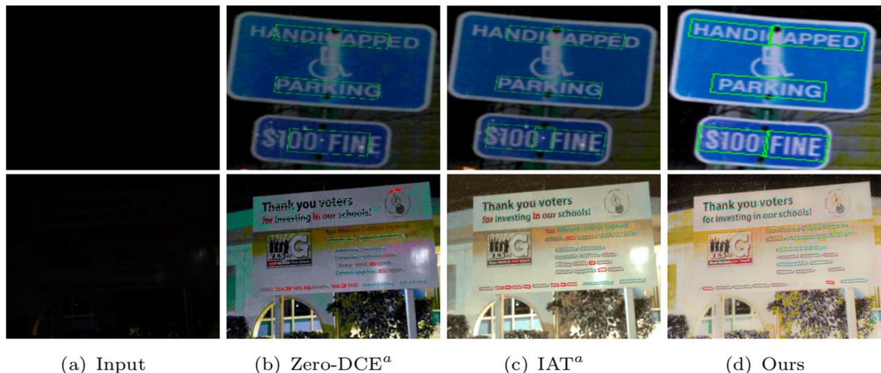
Fig. 7 Vision comparison of text detection algorithms on different low-light image enhancement methods. a represents that the model was pre-trained in the enhancement phase
