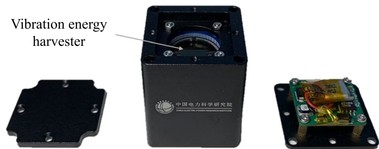
Fig. 6 Photograph of vibration energy harvester with package shell
