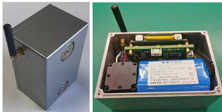
Fig. 15 Photographs of the self-powered vibration monitor for transformers
