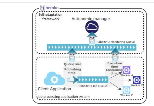
**Figure 4 Prototype architecture.** The prototype architecture used in our proof-of-concept use-case scenario involves real-time monitoring of service performance by an Autonomic Manager. The Autonomic Manager responds to critical situations at the PaaS level by identifying when 'slow' services should be replaced by faster alternatives.
