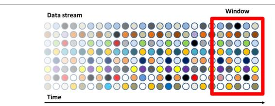
**Figure 2 Querying of streamed data.** Continuous query languages address the problem of querying an unbounded data stream by focussing on a well-defined window of interest.
