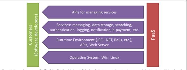
**Figure 1 General structure of a Cloud Application Platform (CAP).** By offering integrated services together with PaaS provision, CAPs reduce the costs associated with complex development.
