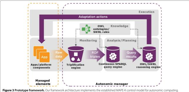
Within the framework, raw data generated by sensors passes through three main processing steps:
