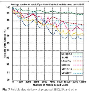
**Fig. 7** Reliable data delivery of proposed SEEQoSA and othe competing approaches with 13,500 mobile cloud users
