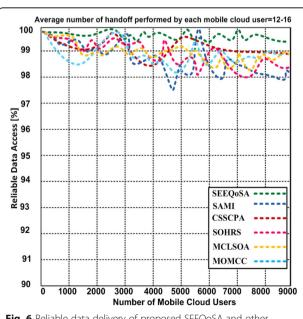
**Fig. 6** Reliable data delivery of proposed SEEQoSA and other competing approaches with 9000 mobile cloud users
