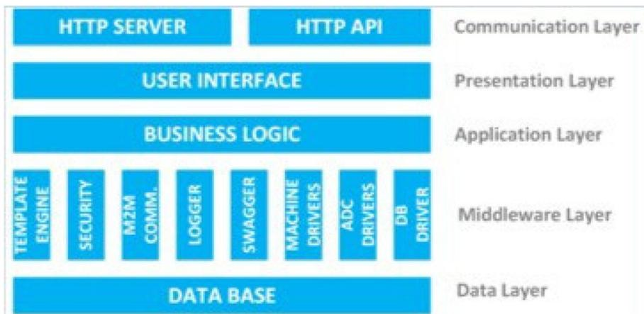
Fig. 5 Machine wrapper (Pi-Wrapper) software architecture
