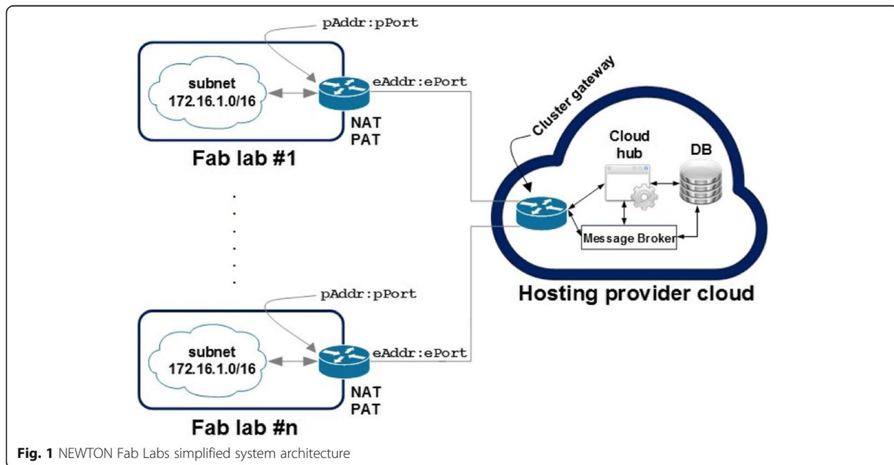
Fig. 1 NEWTON Fab Labs simplified system architecture
