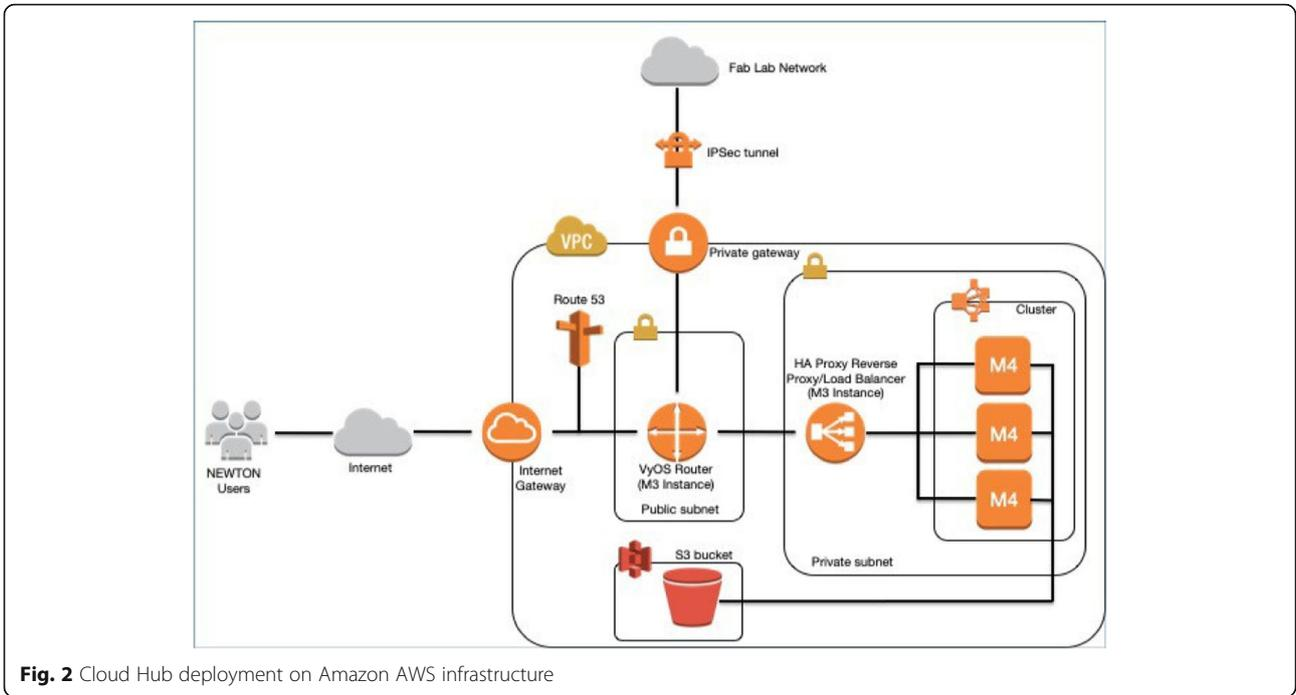
Fig. 2 Cloud Hub deployment on Amazon AWS infrastructure
