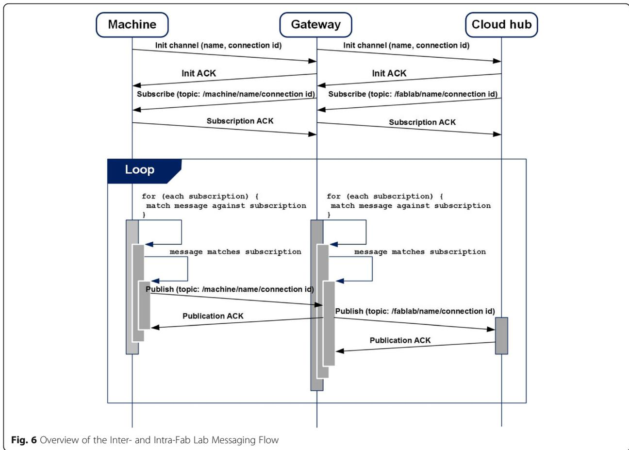
Fig. 6 Overview of the Inter- and Intra-Fab Lab Messaging Flow
