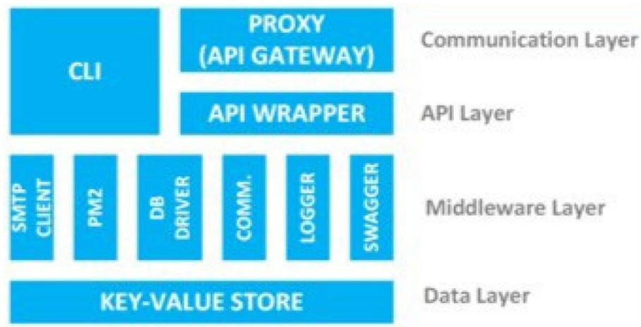
Fig. 4 Fab Lab Gateway (Pi-Gateway) software architecture
