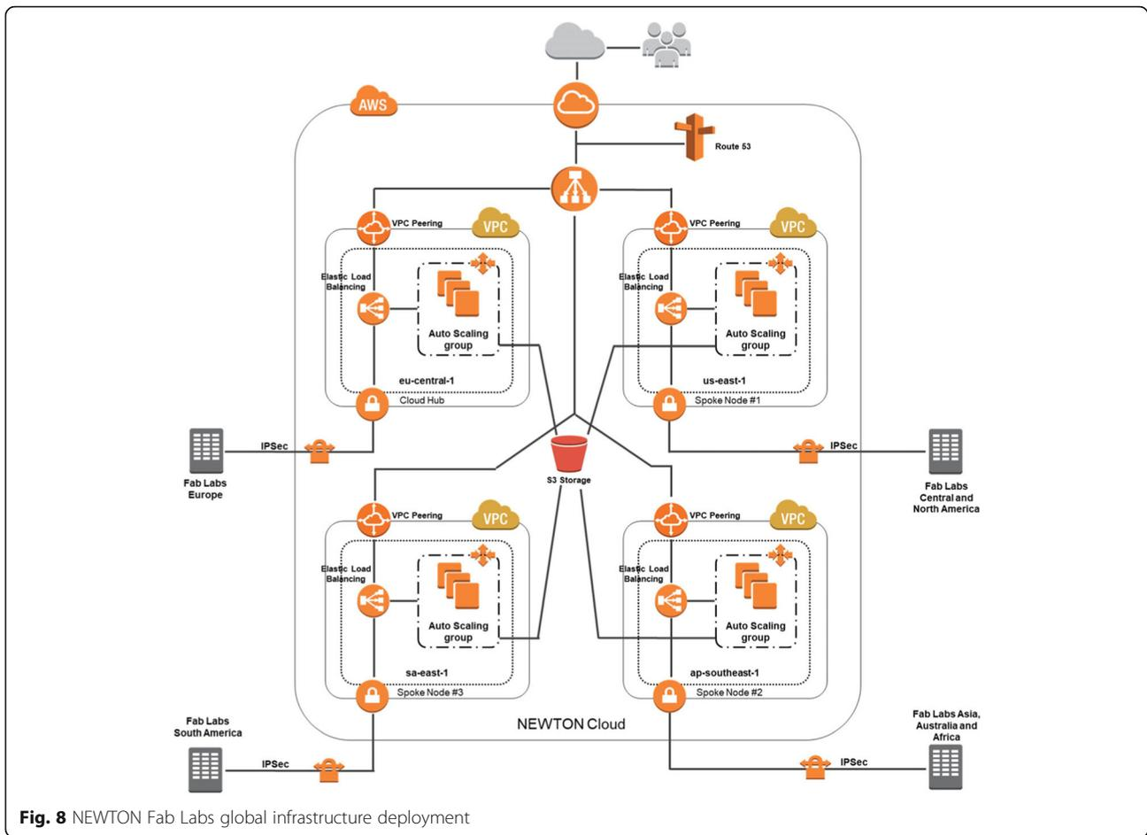
**Fig. 8** NEWTON Fab Labs global infrastructure deployment
