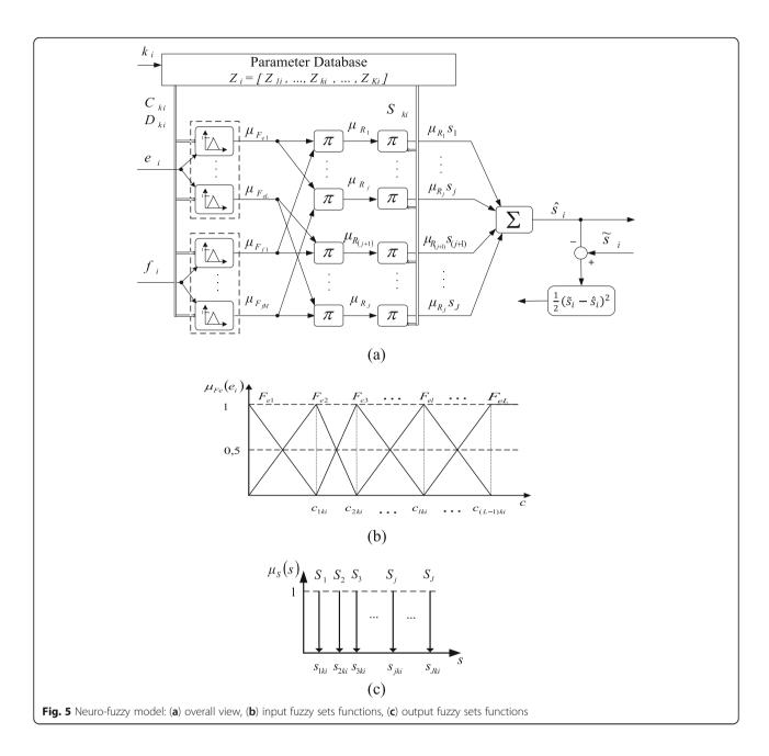
In the preliminary experiments, the optimal value of the number of input fuzzy sets has been determined as L = M = 10, and the number of output fuzzy sets is equal to  $J = L \cdot M$ .
