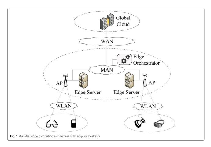
(WAN). The first tier is edge device layer, which is composed of a large number of mobile devices, IoTs and other edge devices. They communicate with local edge server via wireless local area network (WLAN). The second tier is edge server layer, which consist of edge servers and the edge orchestrator. Edge servers are interconnected through MAN. The third tier is cloud server layer, which is the global cloud server distributed around world and provide cloud service through WAN.
